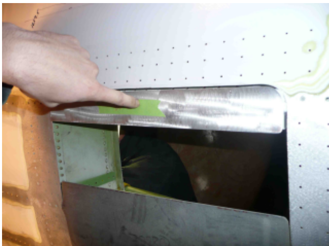
Figure 8. Showing filler panels fabricated to match skin thickness.
